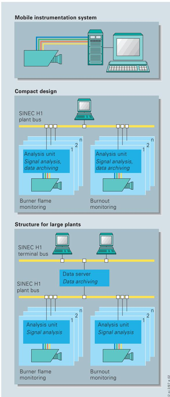
**Fig. 5** Thanks to its highly modular design, the combustion diagnostics system has a wide range of applications from the smallest system for monitoring one burner up to a large-scale system for monitoring an entire boiler, and can be easily integrated into existing process control systems.
